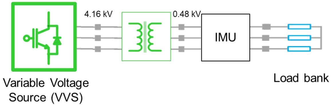
Figure 13. Test setup for low-voltage AC impedance measurement
