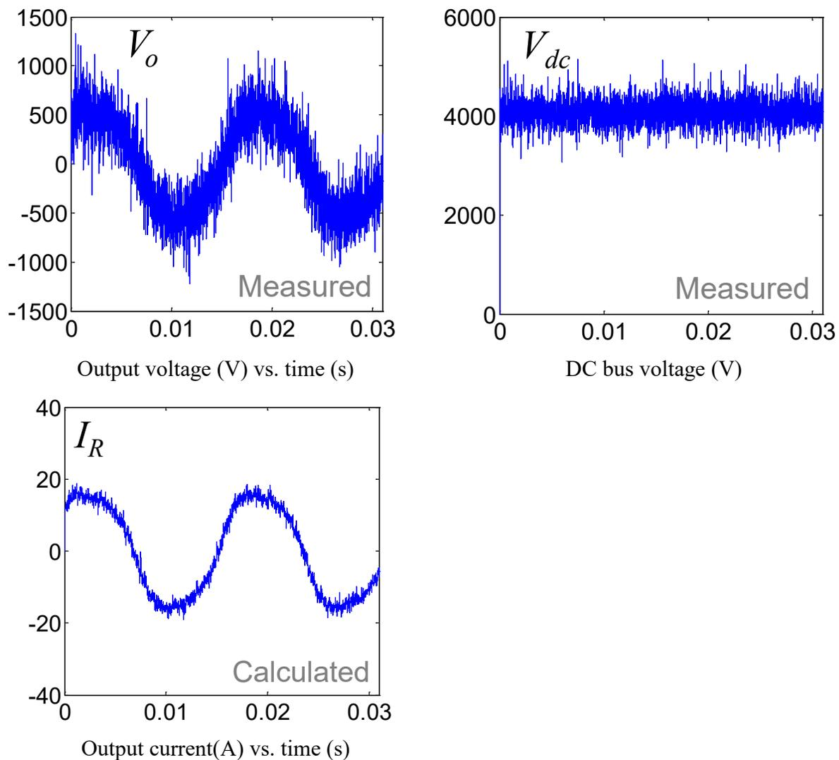
Figure 7. Buck-mode operation: voltage and current waveform captures
