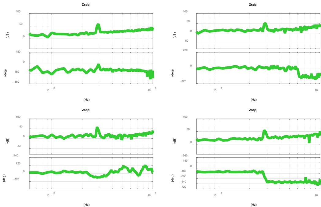
Figure 12. Source impedance measurement result (2.5 kV, resistive load, series injection)
