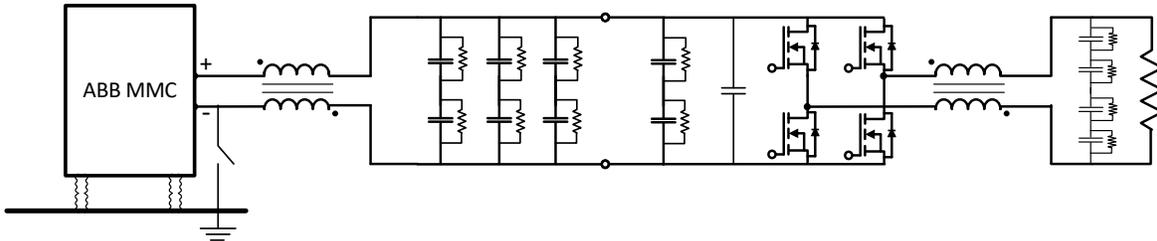
Figure 4. PEBB module testing with H-bridge structure: Supplied by MVDC with grounding option, input and output filters
