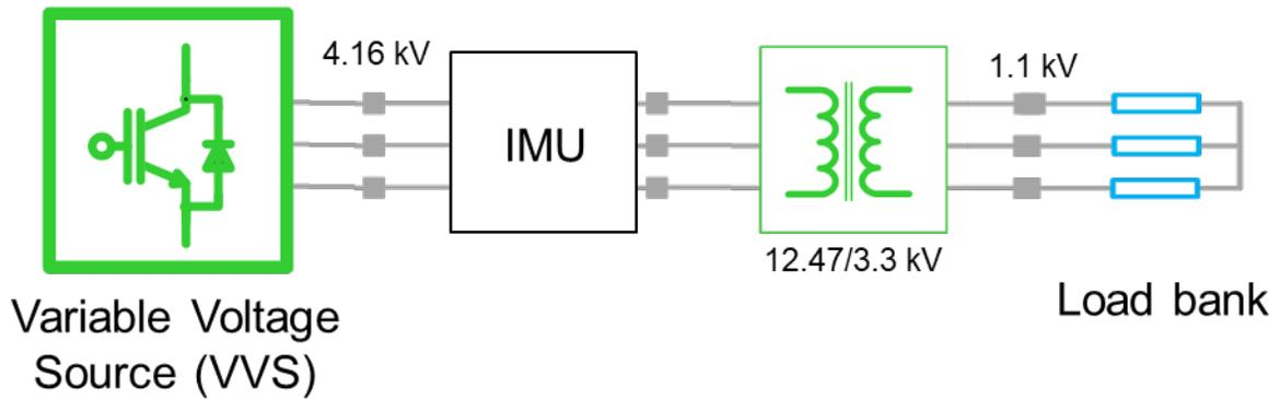
Figure 14. Test setup for medium-voltage AC impedance measurement
