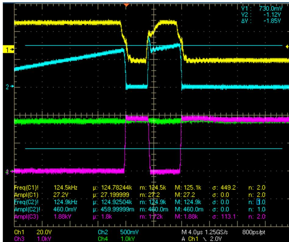
Figure 6. PEBB-Module double pulse test (example capture)
