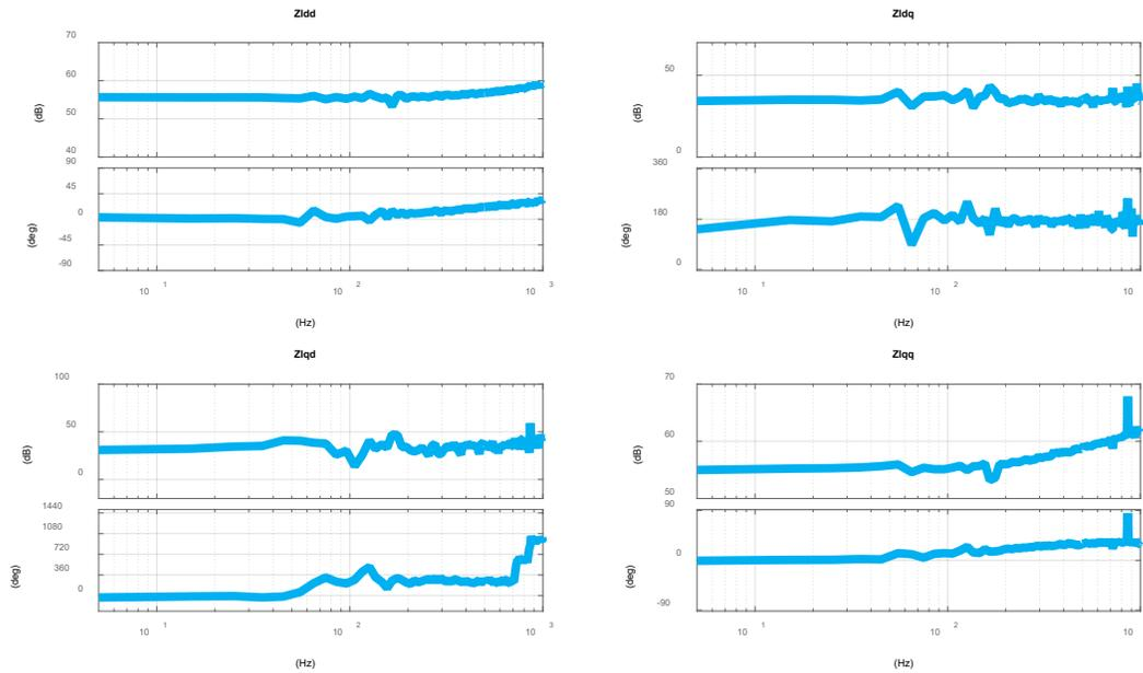
Figure 9. Load impedance measurement result (2.8 kV, resistive load, shunt injection)
