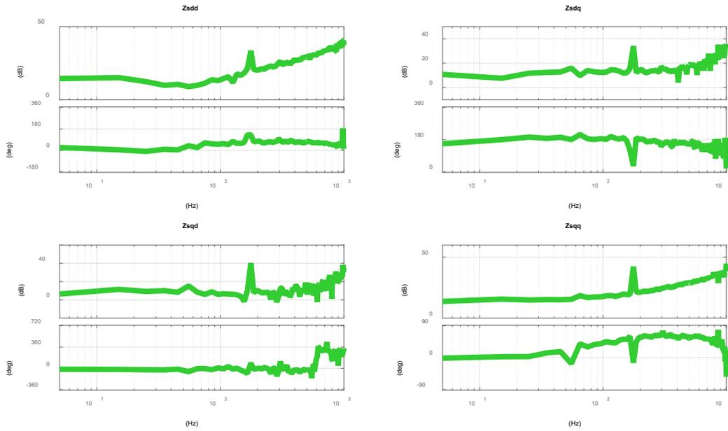
Figure 11. Source impedance measurement result (2.8 kV, resistive load, shunt injection)
