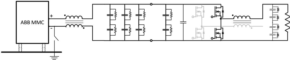
Figure 3. PEBB module testing in buck-mode: Supplied by MVDC with grounding option, input and output filters
