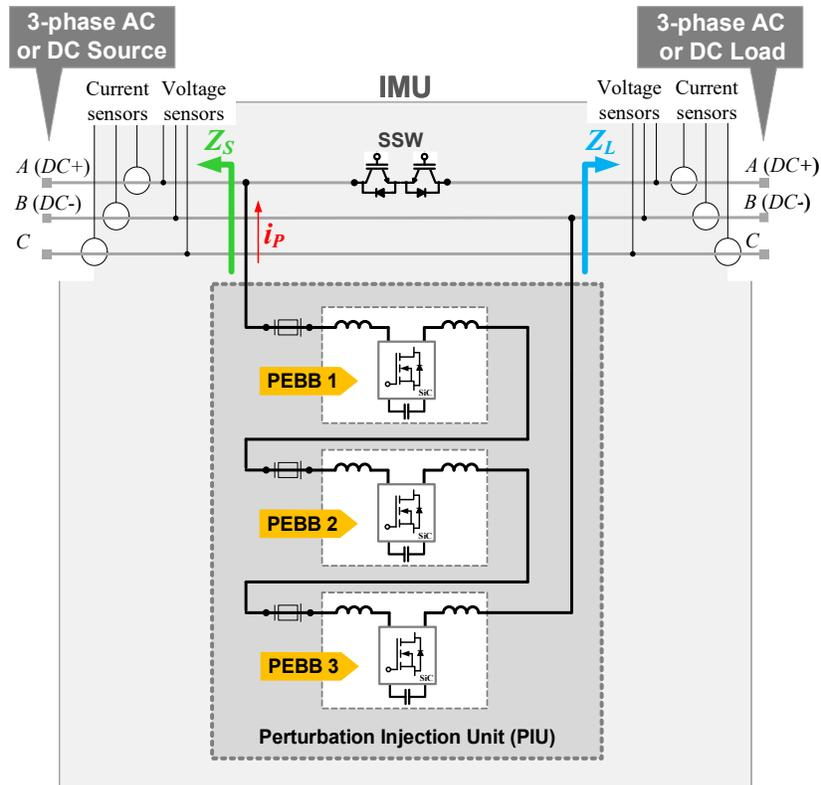
Figure 5. IMU shunt injection mode configuration
