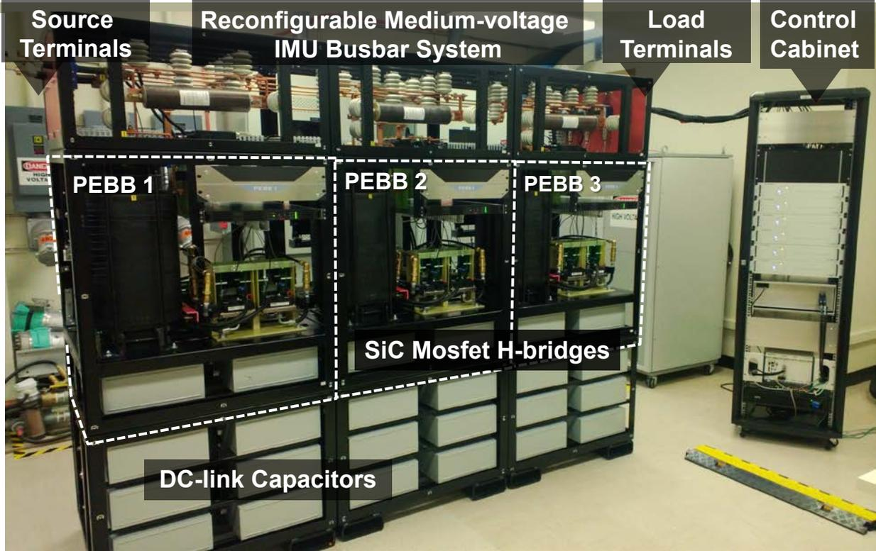
Figure 2. Impedance Measurement Unit
