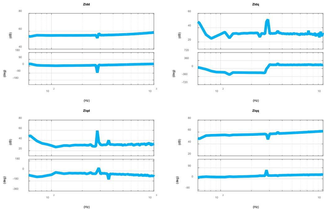
Figure 10. Load impedance measurement result (2.5 kV, resistive load, series injection)
