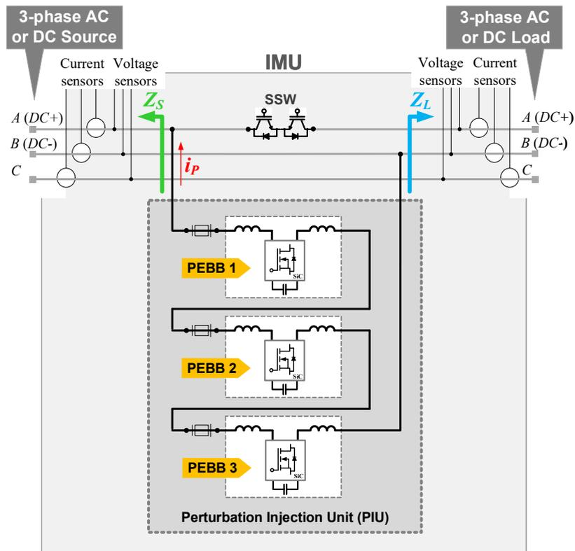
Figure 5. IMU shunt injection mode configuration
