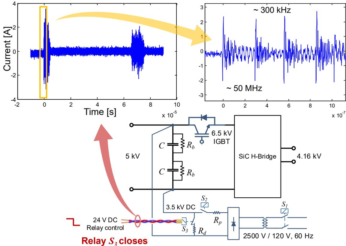
Figure 17. Common mode current triggering DC-bus discharge relay
