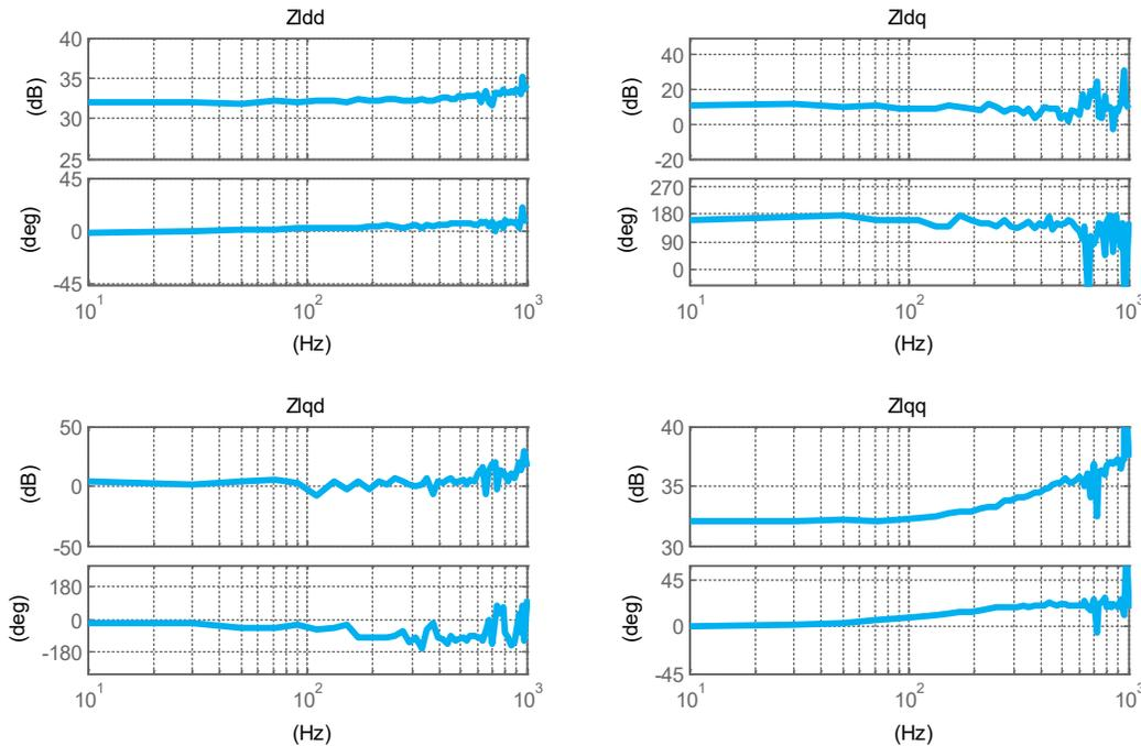
Figure 8. Load impedance measurement result (low voltage, resistive load case)
