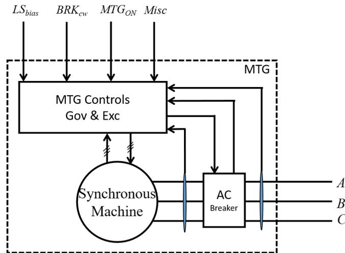
Figure 2.1: MTG Components and Interface
