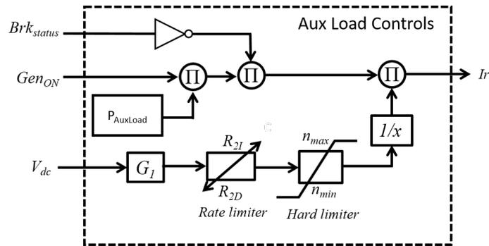
Figure 2.30: Generator Auxiliary Load Controls
