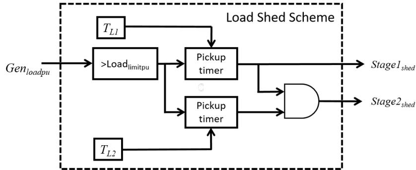
Figure 2.7: Load shedding scheme logic
