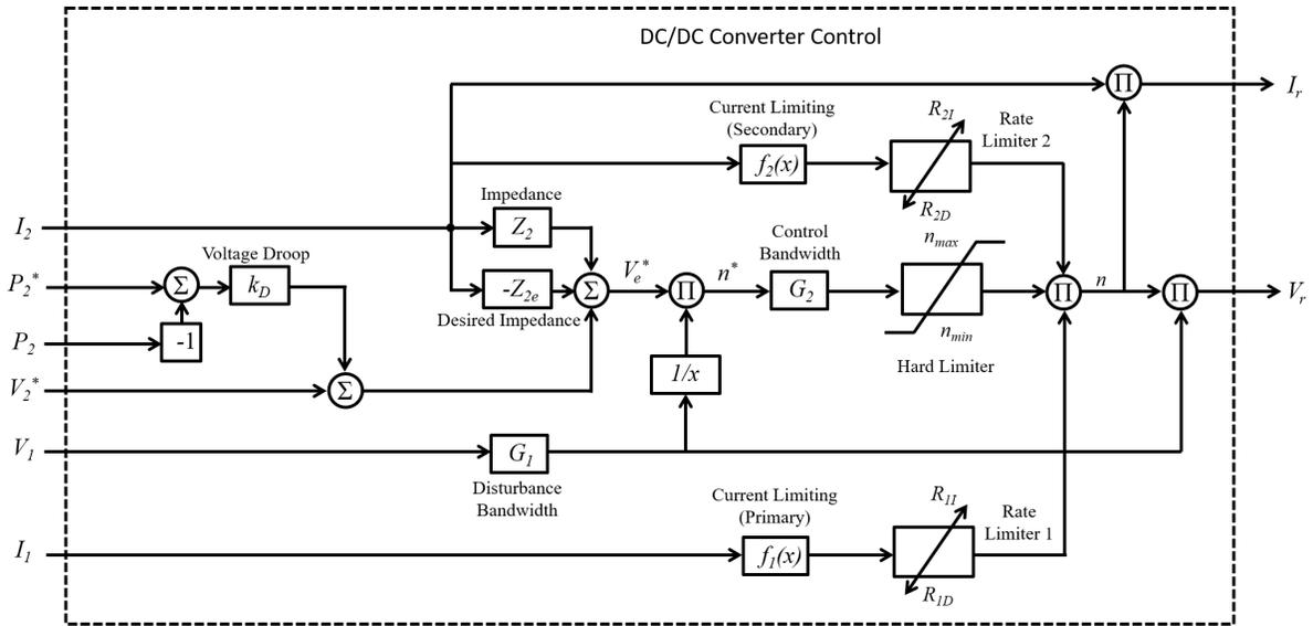
Figure 2.13: Model for DC/DC Converter Control [1]
