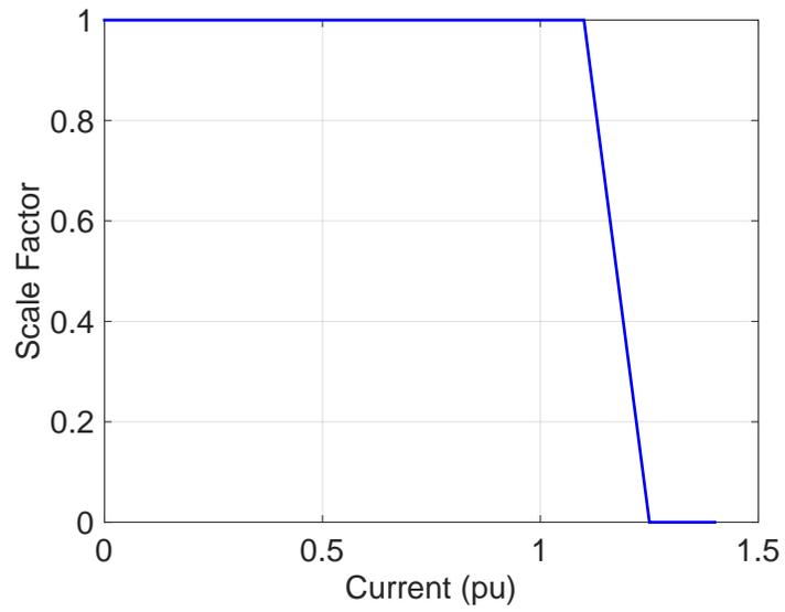
Figure 2.11: Scale Factor Function Current Limiting
