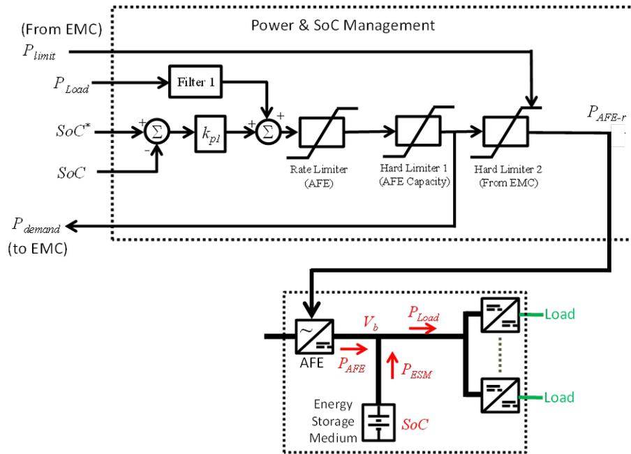
Figure 2.8: Energy Magazine, Power and SoC Management Controls, and Interface to EMC
