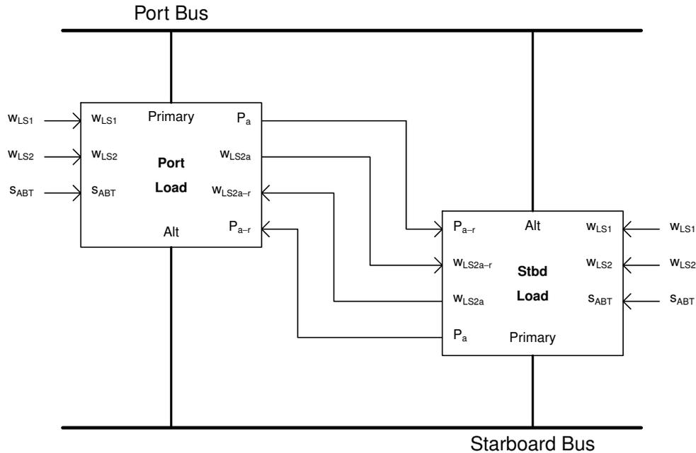
Figure 2.27: Use of Counterpart Load Modules to Represent the Loads within a Distribution Zone
