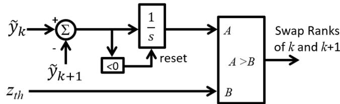
Figure 2.19: Logic for Swapping Rankings of Elements  $k$  and  $k + 1$
