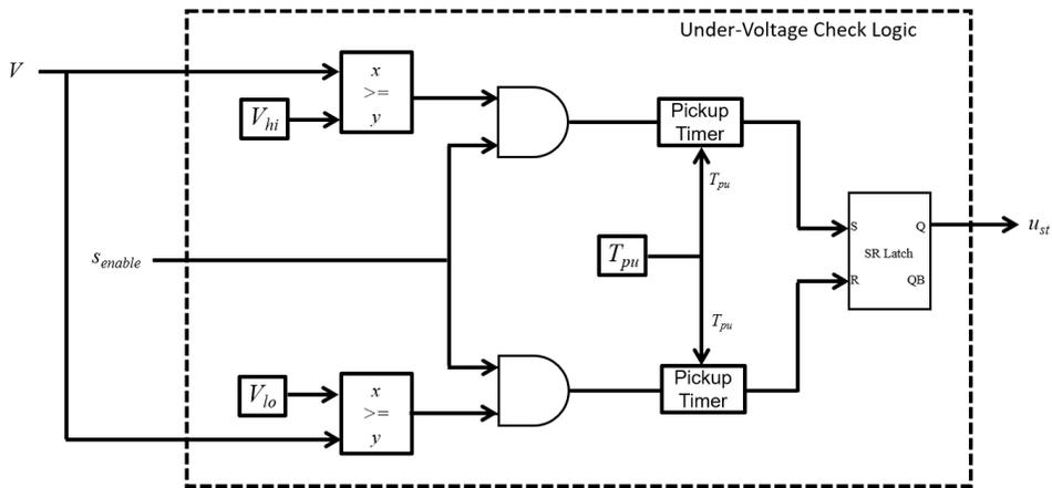
Figure 2.25: ML Under-Voltage Check Logic
