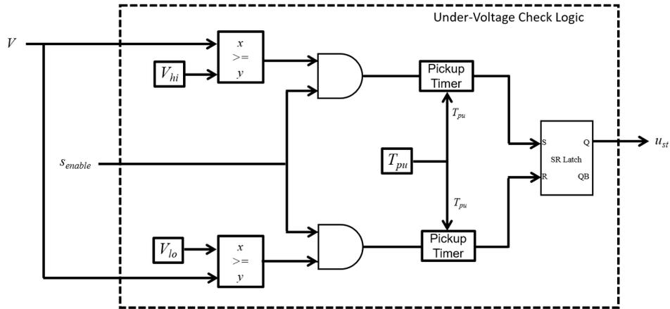
Figure 2.22: PMM Under-Voltage Check Logic
