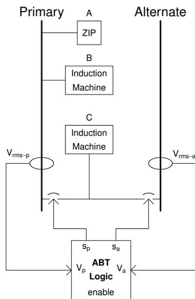
Figure 2.26: Basic Implementation of Aggregate Load Model
