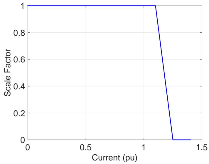
Figure 2.14: Scale Factor Function Current Limiting
