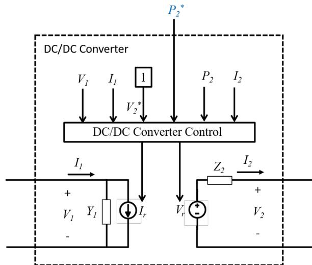
Figure 2.12: Model for DC/DC Converter [1]
